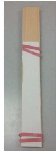
Figure 3: Water Depth Measurement Device
